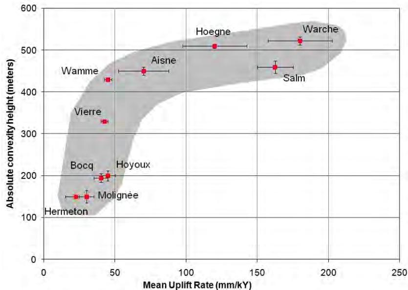
Figure 4. Relation between the  $MUR$  and the  $Cha$  parameters for the selected catchments. Errors bars are represented according to the position of the uplift isolines inside the catchment and to the position of the knickpoint into the longitudinal profile.
