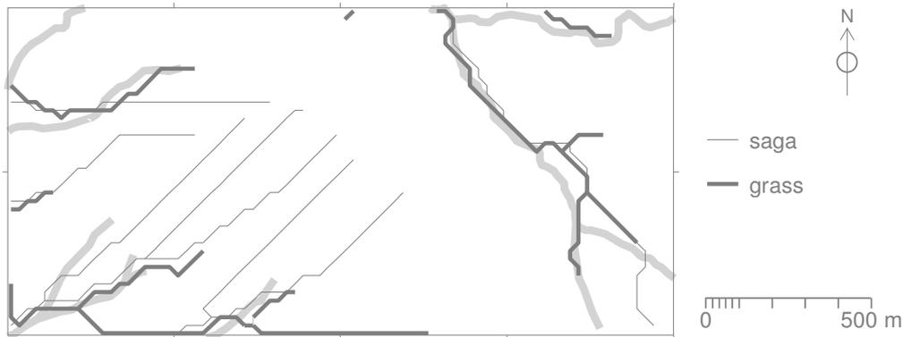
Figure 2. Hydrological networks extracted using the 1 arcsec SRTM DEM (DEMSRTM1.asc) dataset in SAGA GIS and GRASS GIS, as compared to stream network digitized from the 1:24k topo-map (grey bold lines).
