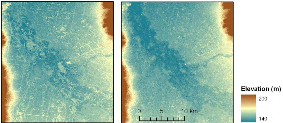
Figure 4. An example of vegetation removal. The elevated linear features are due to trees along roads, while the larger elevated features are patches of forest among cleared land. Most of the offsets are completely removed, revealing the inset floodplain of the river flowing through the centre of the image.
