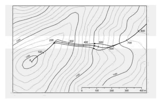
Figure 2. Flow lines derived from a 20 m resolution DLSM
