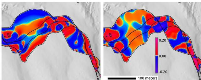
Figure 6. Curvature in the direction of the fastest temporal change (left) and in the perpendicular direction (right) derived from the spatio-temporal surface of 12 m contour evolution.
