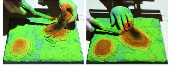
Figure 2. Physical laboratory terrain model at the initial and final state with projected elevation color map and contours derived from the model scan using Tangible Landscape [6].
