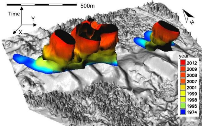
Figure 1. Jockey’s Ridge dune: lidar based DSM (year 2009) and an isosurface showing evolution of 16 m contour for years 1974 through 2012.
