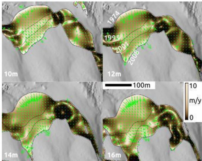
Figure 5. Migration speed and direction for north east part of Jockey's Ridge main dune at elevations 10, 12, 14, and 16 m, derived from the 1974, 1995, 2001 and 2008 DEMs.
