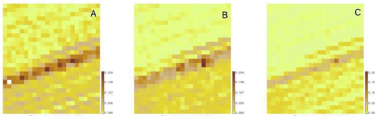
Figure 2. Three different roughness indicators: A standard deviation of DEM, B standard deviation of prominence and C standard deviation of residuals.
