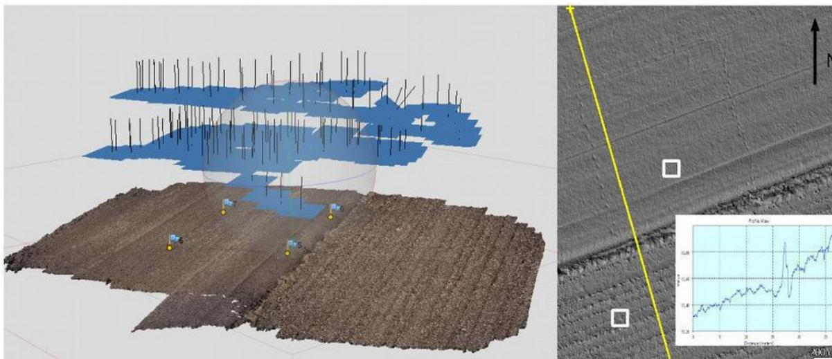
Figure 1. Aerial photos layout (blue rectangles) with generated point cloud (left) and shaded relief with transaction showing height above sea level(right) Examples of area for roughness indices calculation are highlighted in by rectangular.
