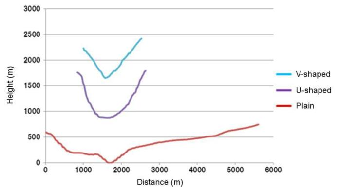
166 Figure 4. Typical examples of three types of valley transverse profiles.
