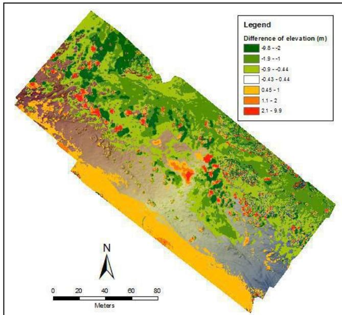
Figure 2. Difference of elevation between the digital surface models of October 2013 and June 2014. Negative values correspond to erosion and positive values to accumulation.
