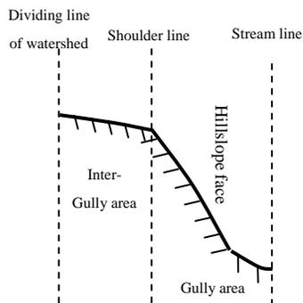
Fig.1 profile structure of hillslope in hilly-gully area
