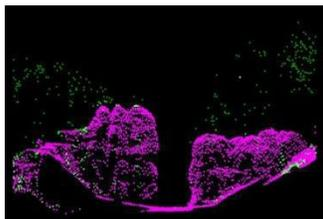
Figure 6. Cross section through correct classified ISOK\_ALS point cloud. (Oct. 2012; 4 pts/m<sup>2</sup>).
