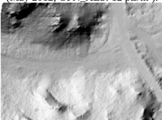
Figure 3. DTM of the "Krakow Gate" in Ojców NP with errors. (May 2012; OPN\_ALS: 12 pts/m<sup>2</sup>).
