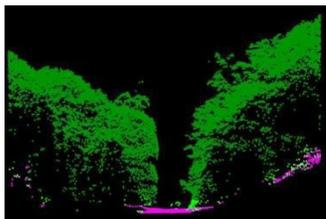
Figure 5. Wrong rock/ground classification. OPN\_ALS point cloud (May 2012; 12 pts/m<sup>2</sup>).
