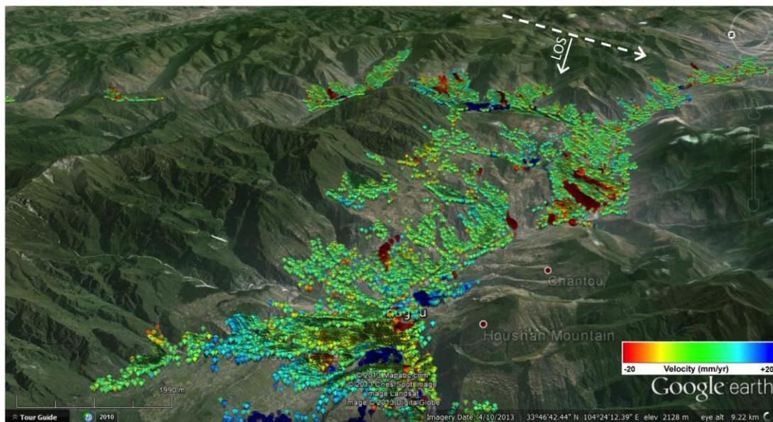
Figure 2. Distribution and average line of sight (LOS) velocity of radar targets in the Southern Gansu Mountains, China. Reddish and bluish dots represent targets moving, respectively, away from and toward the satellite sensor. The high density of targets, especially along the Bailong River valley, allowed the detection of numerous, large active landslides with average displacement rates exceeding 100 mm/year. The background image is from Google Earth™.
