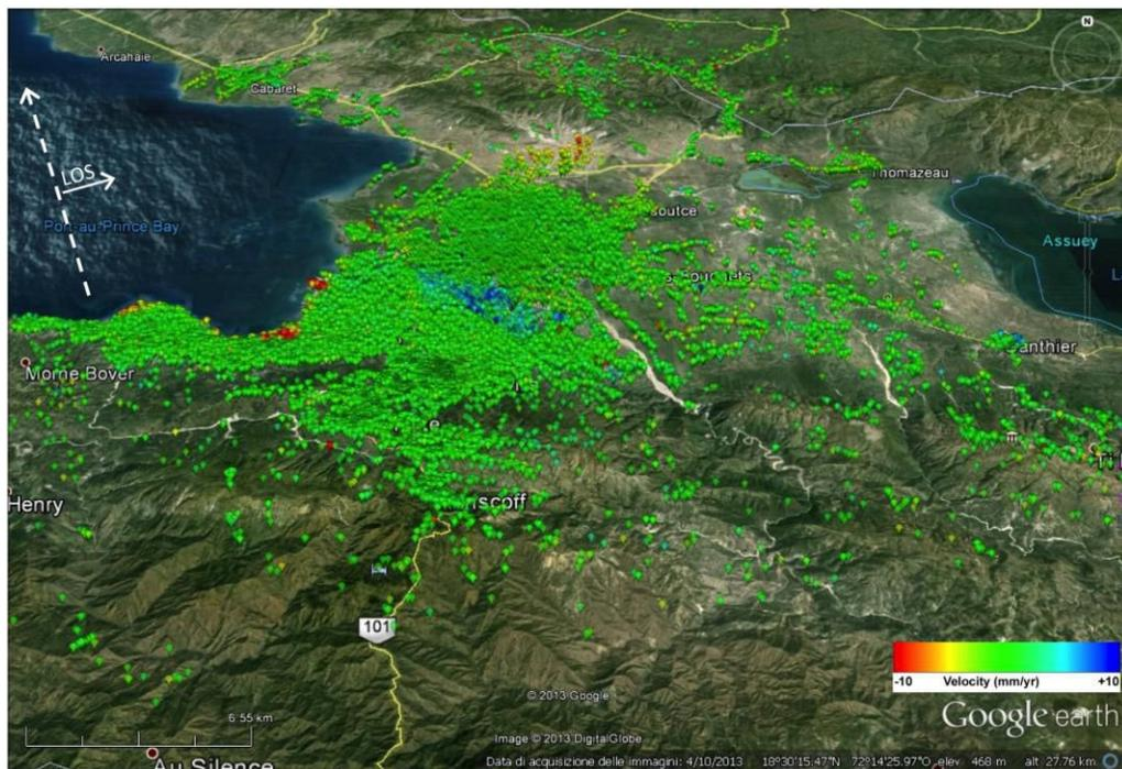
Figure 1. Distribution and average line of sight (LOS) velocity of radar targets (color dots) identified in the metropolitan area of Port-au-Prince, Haiti, and the surrounding regions; the targets are mainly human-made structures, rock outcrops, bare ground). Reddish to yellowish dots represent targets moving away from the satellite sensor and denote significant (up to few cm/year) subsidence affecting coastal areas. The background image is from Google Earth™.
