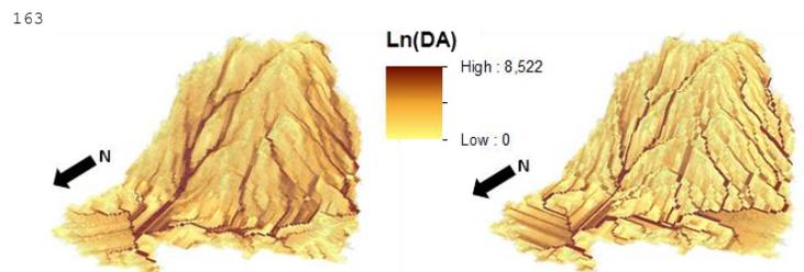
Figure 1. Map of Ln(DA) using the triangular form-based (left) and the single algorithm (right). For each grid-cell, the value 1 is added before calculating the natural logarithm. The map is draped on a digital elevation model (enhanced five times).
