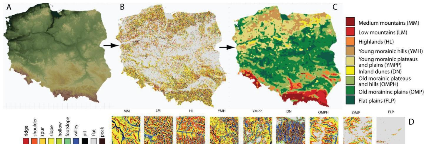
Figure 2. (A) DEM of Poland with 30m resolution. (B) Ten-categories map of landform elements with 30m resolution. (C) Results of pattern-based supervised classification of grid-of-scenes into nine physiographic units. (D) Examples of characteristic patterns of landforms for the nine physiographic units.
