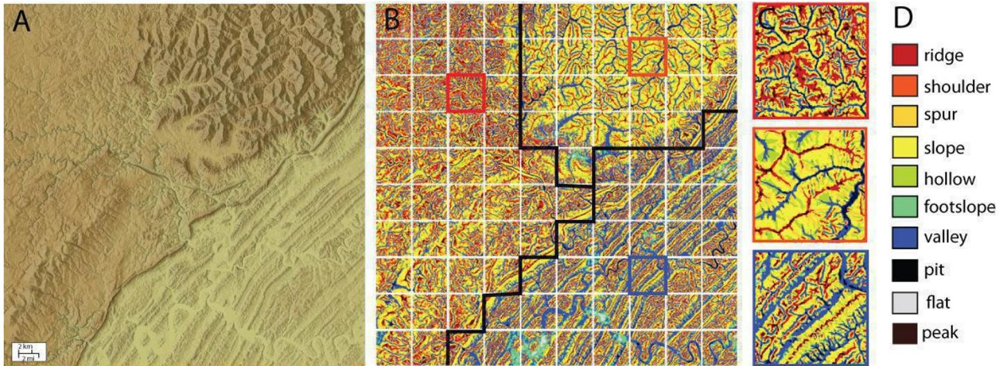
Figure 1. (A) Hillshade rendition of the 2000×2000 cells DEM. (B) Cell-based classification of the DEM into ten landform elements and its sub-division into a grid-of-scenes. (C) Examples of three scenes representing three different physiographic regions present in the region. (D) Landform elements legend.
