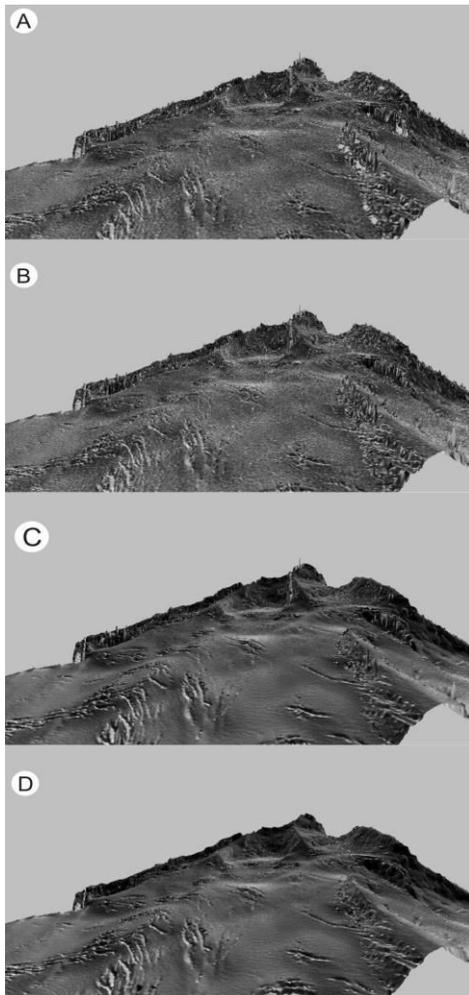
Figure 2. 3D view of Pléiades DEM in the Tronador area shown as a hill shade model: A) without post-processing (note the presence of gaps, granular noise and spikes); B) First step in post-processing, Pléiades DEM with gaps filled; C) Second step in post-processing, Pléiades DEM with speckle noise removed; D) Final Pléiades DEM without spikes, granular noise and gaps. Note the smoothness of ice surface and how well the crevasses are represented.
