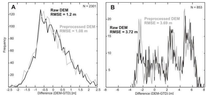
Figure 3. Histograms of differences between DEMs and GTD for Tronador (A) and Vallecitos (B) areas. Thick black line represents the error distribution of the raw (non processed DEM), grey line represents the error distribution of post-processed DEM.
