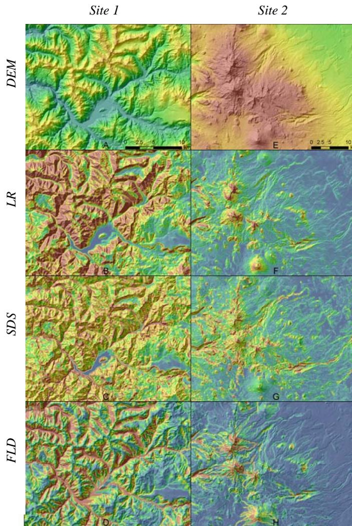
Figure 2. A, E: DEM with hillshade (resolution = 37.2 m); B, F: Local Relief (*LR*) with hillshade; C, G: Standard Deviation of Slope (*SDS*) with hillshade; D, H: Flow-Length Difference (*FLD*) with hillshade. Warm color indicates high value.
