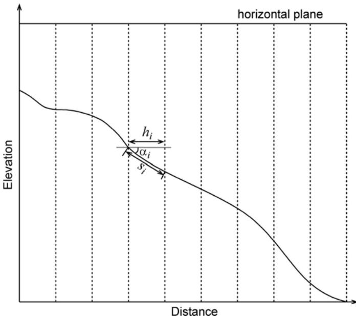
Figure 1. Schematic diagram showing a profile along a flow path.  $s_i$  is the 3D flow length along topographic surface at the  $i$ -th cell;  $h_i$  is the projected horizontal flow length at the  $i$ -th cell;  $\alpha_i$  is the local slope at the  $i$ -th cell. (distances between each vertical dotted lines are either the same as cell size or 1.41 times the cell size)
