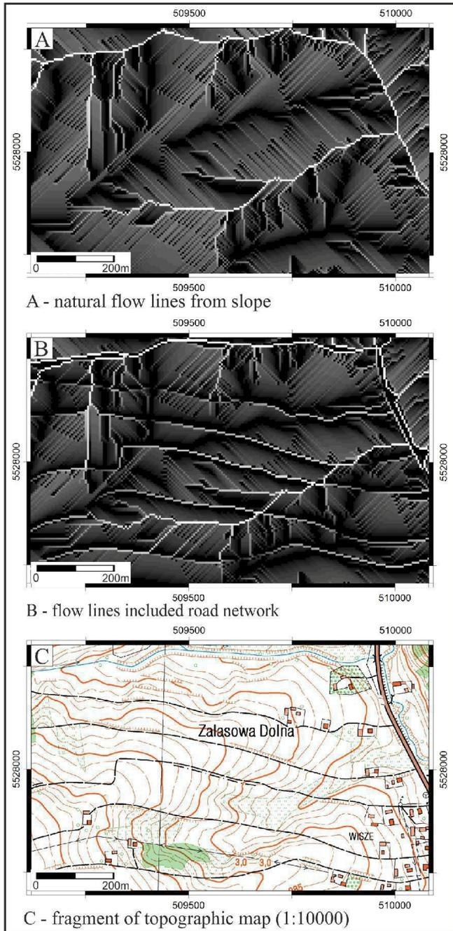
Figure 2. The natural – A and modified – B by road networks surface drainage systems in a part of the Zalasówka catchment. The lowermost part – C presents the topographical map of this area.
