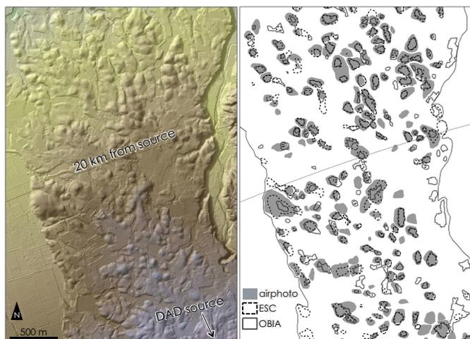
Figure 1. Hillshade image of the central part of the study site by 2-m resolution airborne laser scanning DEM, and hummock polygons extracted by the three different methods; light-gray-filled: manual airphoto reading, dashed black outline: ESC; solid dark-gray outline: OBIA
