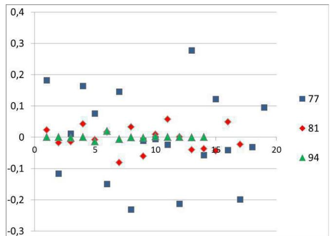
Figure 3. Vertical dispersion of the control points residuals; X axis presents number of the control point, Y axis scaled in metres.
