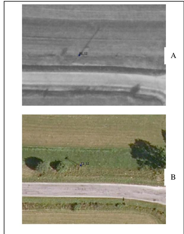
Figure 1. Example of location of a control point on the low voltage pole basis; A – aerial photo of 1981, B – orthophotomap of 2009.
