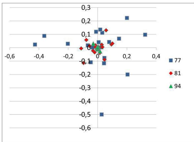
Figure 2. Horizontal dispersion of the residuals of the control points for each air raid. X and Y axis scaled in metres.
