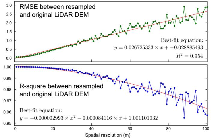
Figure 3. RSME (top) and R-squared (bottom) plots between resampled models and LiDAR data for the Garopaba dune field. Red line shows best fit of first order for RMSE values and of second order for R-squared values.
