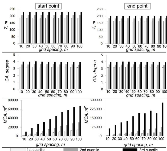
Figure 4. Quartiles for sets of morphometric variables on DEMs with different grid spacing for the dataset of start points and end points on Hronská pahorkatina Hill Land. Left – values for start point of gullies, right – values for end points of gullies, Z - altitude, GA – slope, MCA – maximal catchment area.
