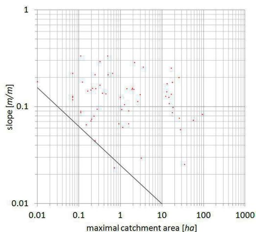
Figure 5. Example of the scatter plot of dependence between maximal catchment area [ha] and slope [m/m] for catchments forested less than 50 % for start (incision) points located in Hronská pahorkatina Hill Land. Each point represents one start point of gully. Gully located below the line is an outlier of the dataset.
