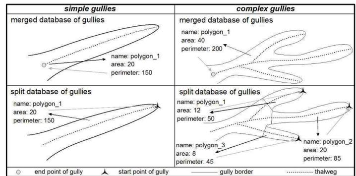
Figure 2. Differences between merged datasets and split datasets in case of simple and complex gullies.
