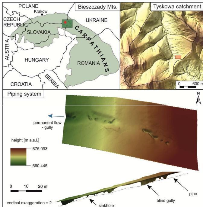
Figure 1. Location of study area with the 3D image of analyzed piping system.
