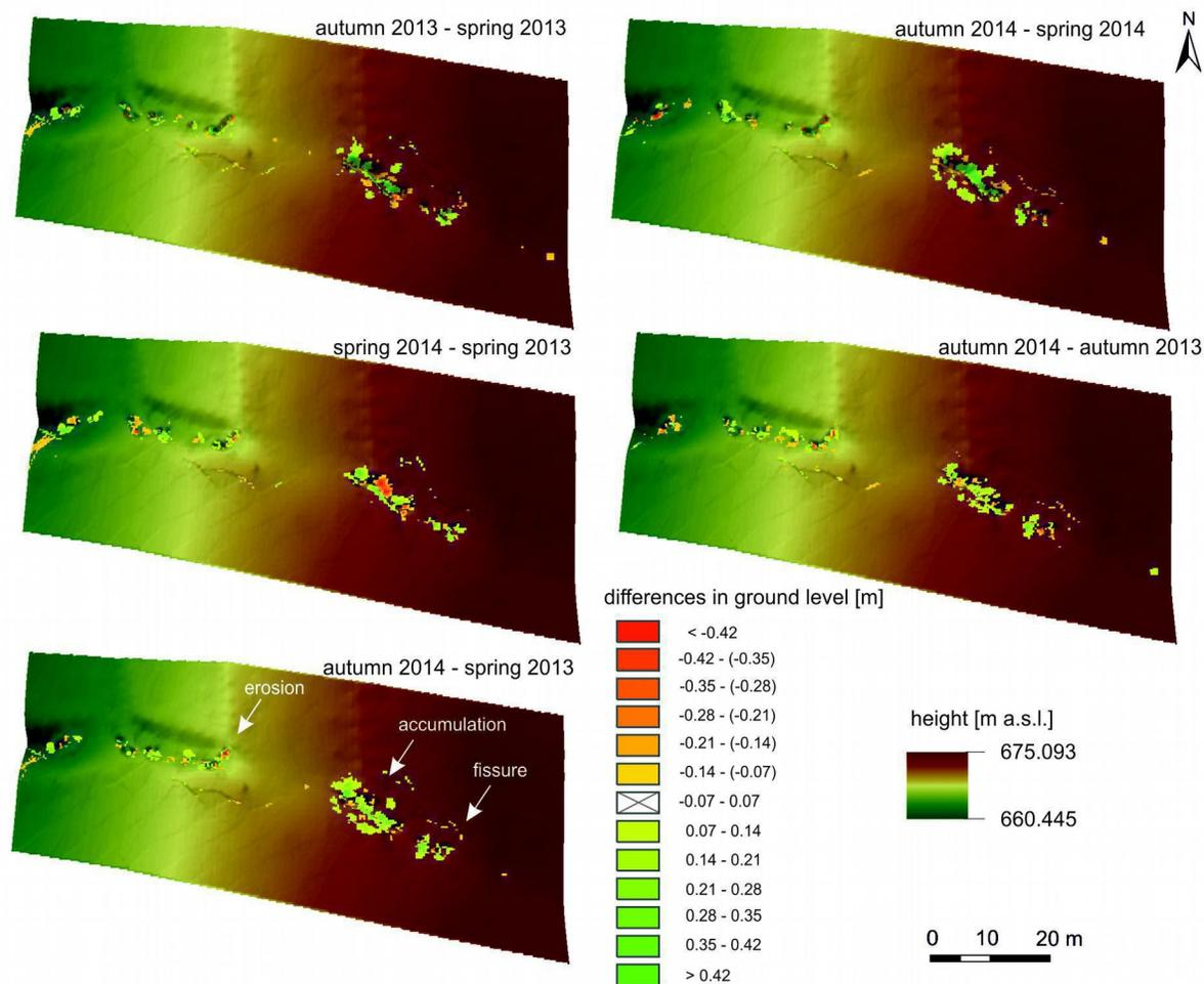
Figure 3. The morphometric changes in the piping system in 2013-2014.
